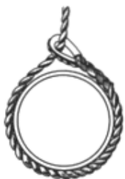
Correct - Use thimbles in the eyes
