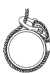
Correct - Shackle pin cannot turn
