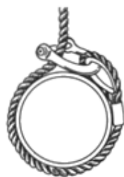
Incorrect - Shackle pin in contact with running line can work loose
