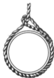
Incorrect - Eye splice may cut running line
