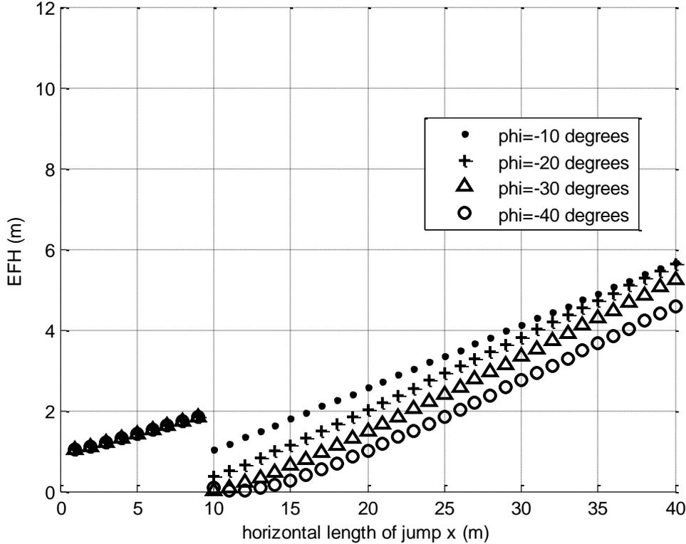
Figure 21. EFH of landing on a downward slope as a function of jump distance  $x$  for several values of  $\varphi$  with constant parameters  $x_t=10\text{m}$ ,  $y_t = 1\text{m}$ , and  $\theta_0=25^\circ$
