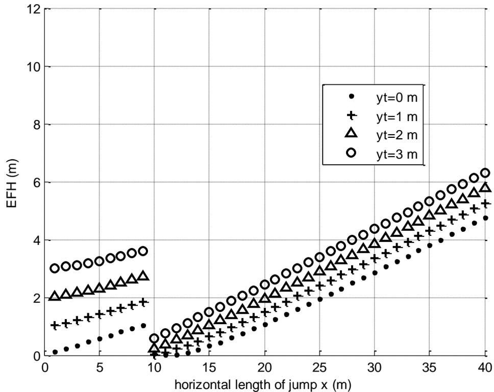
Figure 18. EFH of landing on a constant downward slope as a function of jump distance  $x$  for several values of  $y_t$  and constant parameters  $x_t=10\text{m}$ ,  $\theta_0=25^\circ$ , and  $\varphi=-30^\circ$
