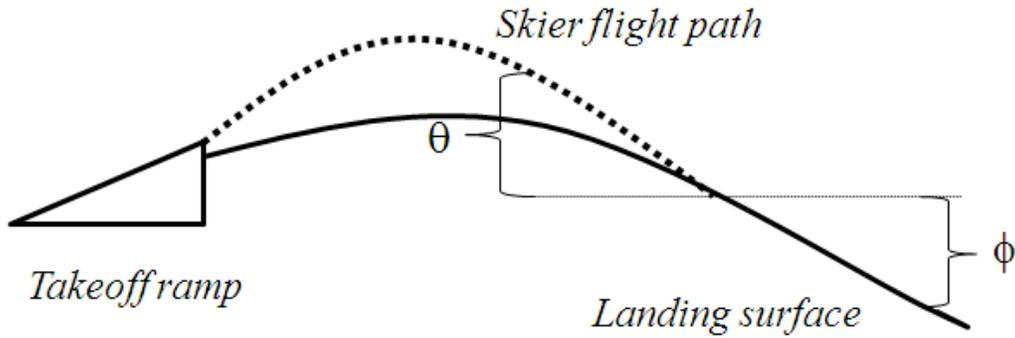
Figure 9. Skier flight path and safe surface design
