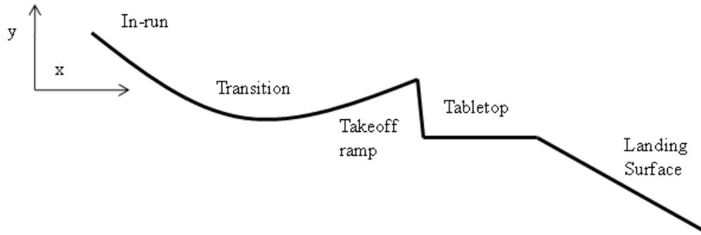
Figure 5. Profile for a typical terrain park jump
