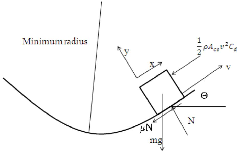
Figure 47. Free Body Diagram for a clothoidal transition
