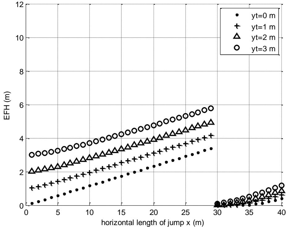
Figure 20. EFH of landing on a constant downward slope as a function of jump distance  $x$  for several values of  $y_t$  and constant parameters  $x_t=30\text{m}$ ,  $\theta_0=25^\circ$ , and  $\varphi=-30^\circ$
