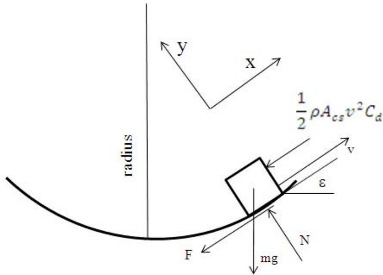
Figure 39. Free body diagram of a particle in the circular transition region
