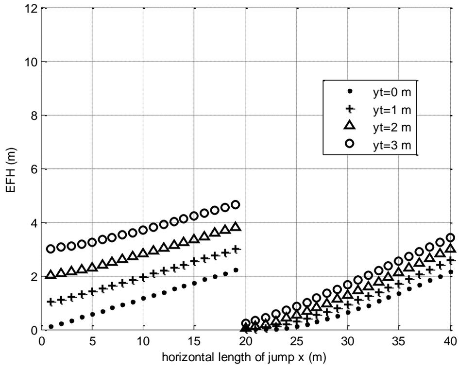
Figure 19. EFH of landing on a constant downward slope as a function of jump distance  $x$  for several values of  $y_t$  and constant parameters  $x_t=20$ m,  $\theta_0=25^\circ$ , and  $\varphi=-30^\circ$
