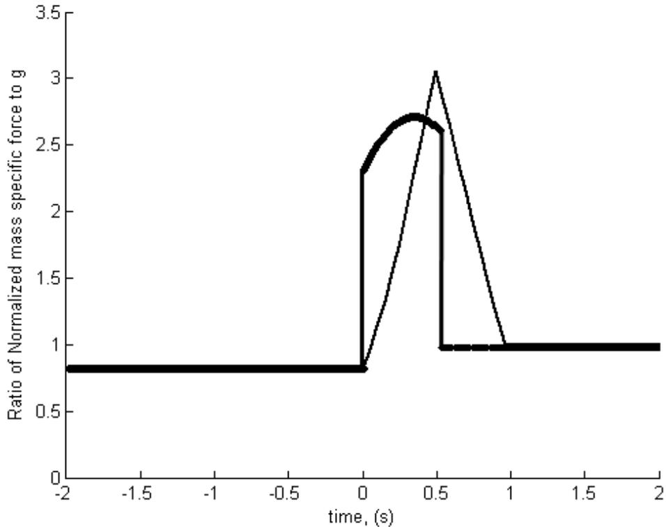
Figure 55. Comparison of the ratio of normal acceleration vs. time for circular and clothoidal transitions in the in-run, transition, and takeoff ramp for  $\lambda = 35^\circ$ ,  $\beta = 10^\circ$ ,  $\mu=0.05$ ,  $\gamma = 1.5$ , and  $C_d = 0$
