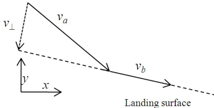
Figure 8. Perpendicular velocity changes upon landing impact
